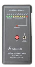
This meter has been designed to measure both surface resistance and resistance to ground. To measure surface material place the meter on the area to be tested and press the test button. For measuring resistance to ground, place the ground lead into the earth leakage socket, connect the crocodile clip to the area to be tested and press the test button.
