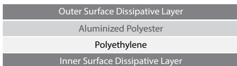
Fig.4. Structure of a Metal Out Shield Bag.
