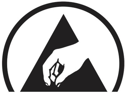
The ESD Protective Symbol consists of the reaching hand in the triangle. An arc around the triangle replaces the slash. This “umbrella” means protection. The symbol indicates ESD protective material.
