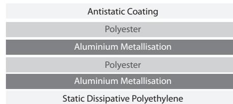
The heavy metallisation structure is essentially that of a shielding bag but with opaque, thick layers of metallisation. Nylon is regularly used in place of Tyvek or polyester, providing the needed strength at a lower cost than Tyvek.
