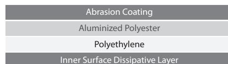
Our bags are manufactured from industry approved polyester and polyethylene laminates. The polyester dielectric works with the metal layer to provide a Faraday effect, the metal layer preventing penetration from damaging electrostatic fields. The specially processed polyethylene keeps tribocharging to a minimum.
