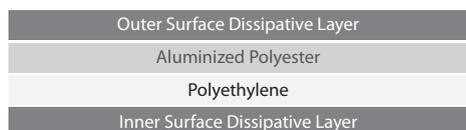
Fig.4. Structure of a Metal Out Shield Bag.
