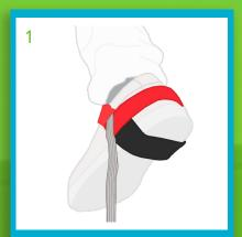
Remove heel grounder from its packaging and place the conductive rubber strip on the heel grip of the shoe
