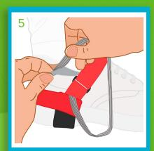
Feed the conductive ribbon into the sock or shoe to complete the grounding path
